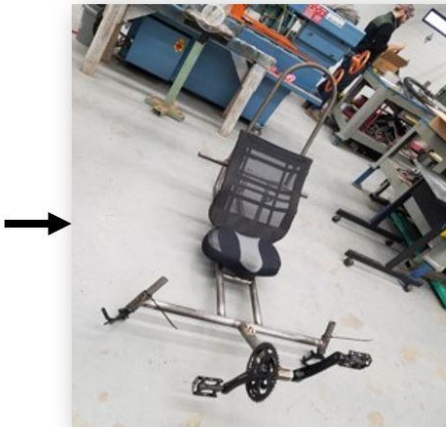
Prototype – January 14, 2019 Crossbar, Head tubes, Steering Knuckles, Pedals
